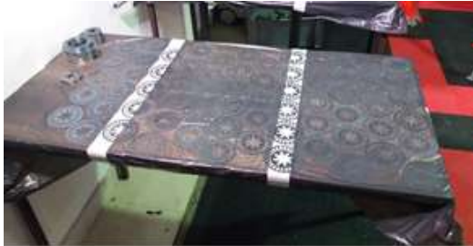
Figure 2.2 - Stator and Rotor sheets with manually applied Epoxy
