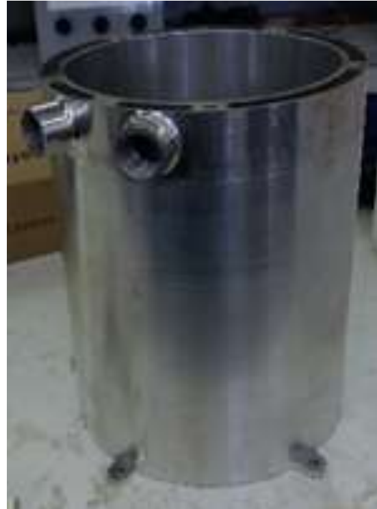
Figure 2.4 - Machined motor housing
