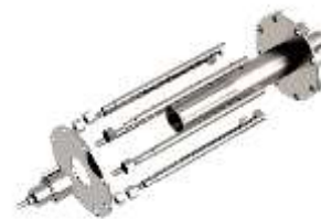
Figure 6.4 - Exploded view of the final shaft version
